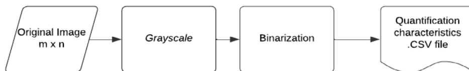
Fig. 1. Flowchart describing the image processing steps and the generated files.
